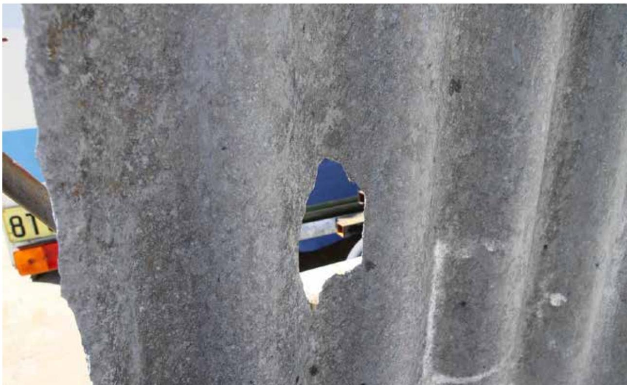
**MIX OF CROCIDOLITE (BLUE ASBESTOS) AND CHRYSOTILE (WHITE ASBESTOS)**
